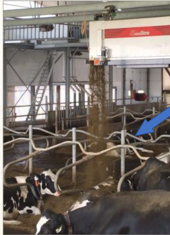
Solids delivered to deep bedded stalls with a track mounted delivery cart
