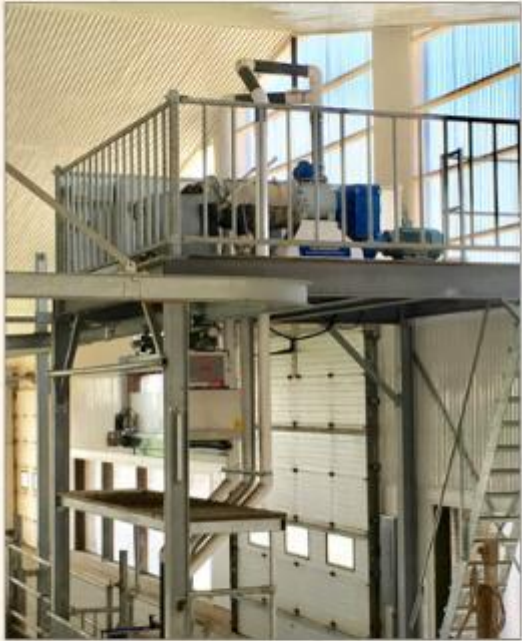
Screw press separates manure solids
