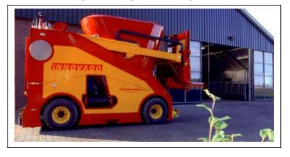
direct the machine to a good cutting position. A face cutter with scales cuts the required amount of each ingredient. Wet by-products are loaded with a platform adaptor on the cutter. Wireless control of augers, doors, unloaders, pumps and valves are used to load product from
